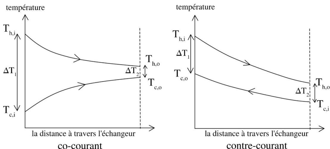
$T_{h,i}$  is the temperature of the hot fluid at the inlet of the exchanger
